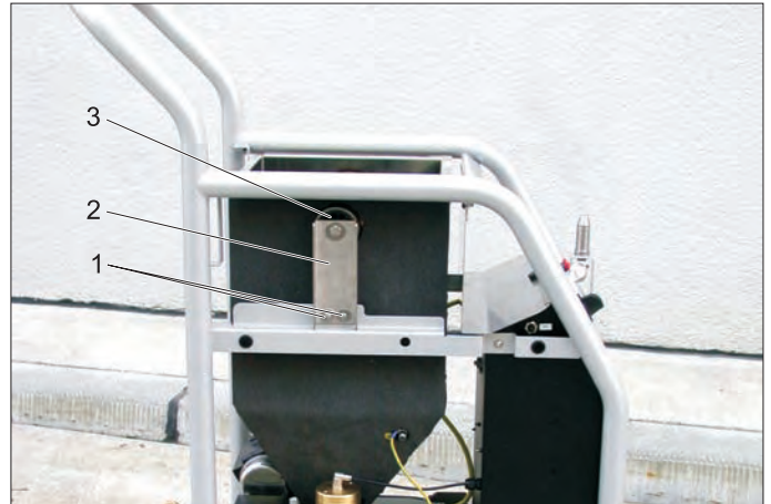
1 Fastening screws for dry ice container support
